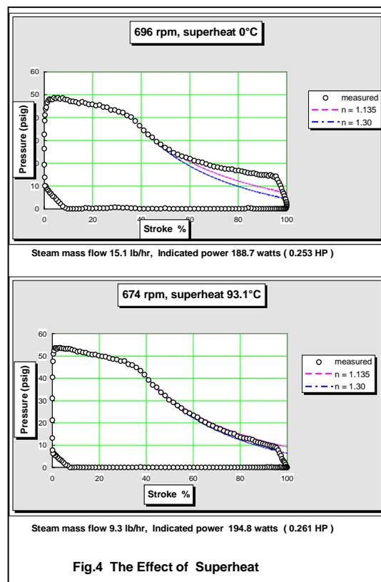
Fig.4 The Effect of Superheat
