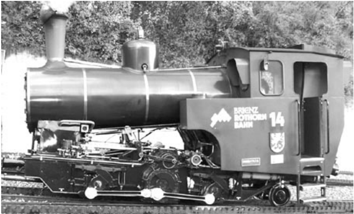
1996-built High Efficiency “Second Generation” Steam Locomotive designed and built for the Brienz Rothorn tourist railway in Switzerland by DLM. The railway purchased five of these locomotives after discovering that they not only attract more tourists, but outperform and are cheaper to operate than diesel railcars.
